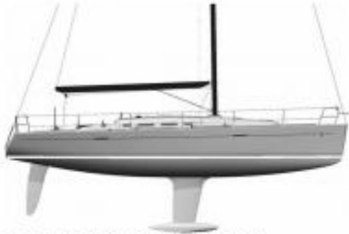
Deep draught keel - Cast iron / Lead (optional)
